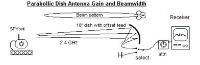
reflector. The increase in aperture area yields a corresponding antenna "gain". As discussed in class, placing a small reflector behind the dipole at the focal point doubles the energy into the dish and minimizes sidelobes, thus adding to the overall gain by about 3 dB.
