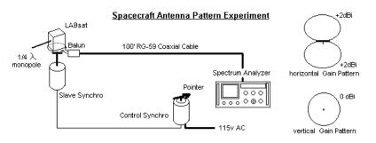
horizontally. Although the monopole antenna on one face of the satellite would appear to give an unbalanced radiation pattern when rotated horizontally, in fact, the pattern will not be that much different from the  $\frac{1}{2}$  wave dipole pattern observed in the EA-204 lab. This is because the ground plane of the spacecraft is small relative to wavelength and simply acts as a counterpoise to reflect the missing half of the dipole.
